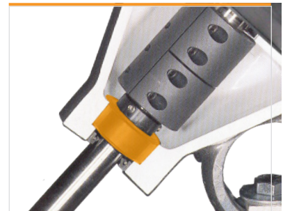
c Auxiliary bearing limits overhung loads on drive
