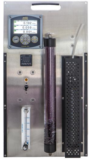
inleakage, makeup water, ion exchange resins, and plant cycle additives. By precise heating of the process solution to near-boiling after a cation column, carbon dioxide and other low molecular organics are volatized and removed providing a degassed cation conductivity measurement that results in a more realistic assessment of the process chemistry.
