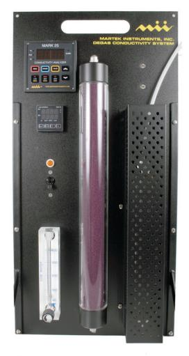
inleakage, makeup water, ion exchange resins, and plant cycle additives. By precise heating of the process solution to near-boiling after a cation column, carbon dioxide and other low molecular organics are volatized and removed. Differential analysis between cation and degassed conductivity measurements provide a more accurate cation conductivity value that can be directly correlated to CO<sub>2</sub> concentration and result in a more realistic assessment of the process chemistry.
