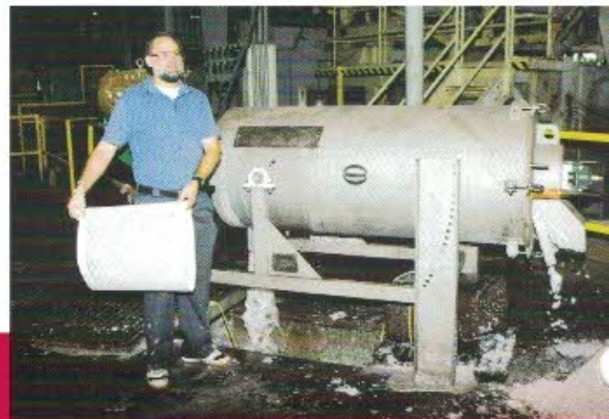
LOW SET ELEVATION FOR HEAVY CAKE DISCHARGE
