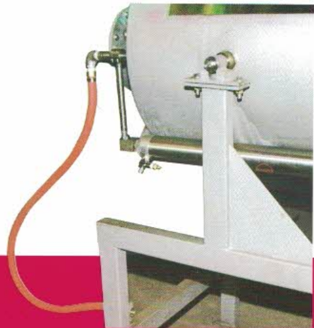
AIR CYLINDER ACTUATOR FOR BACKFLUSH SPRAY
