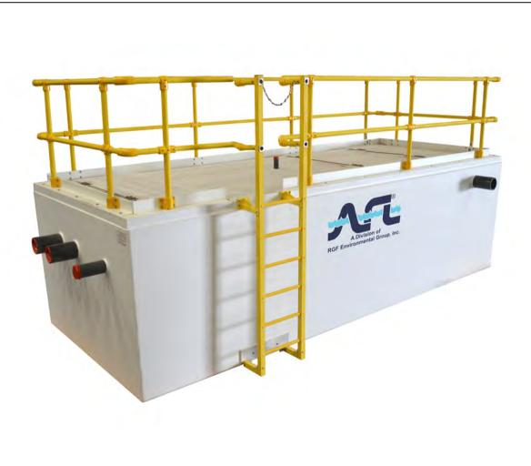
The EGS separates heavy solids and oil from industrial wastewater and storm water using gravity separation. Heavy settleable solids drop out of oily wastewater in the inlet chamber. In the separating chamber, the oil rises and lighter settleable solids fall. Floating oil collected in the separating chamber is collected by a rotary pipe skimmer for collection and disposal. A sheen baffle retains residual floating oil as the treated effluent discharges through the outlet.
