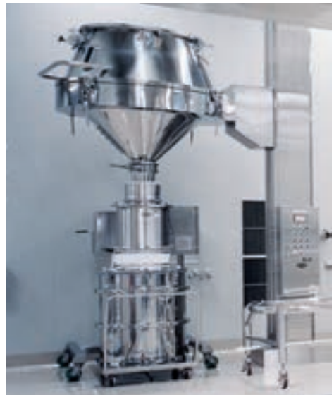
An inverted fluid-bed dryer bowl directly discharges into a Comil® U30 on a portable stand, feeding a stainless steel drum.
