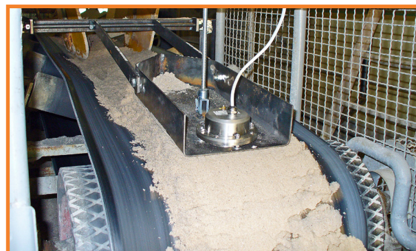
Measuring moisture of sand
