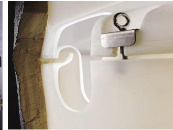
Inner tank's unique dome interlocks with outer tank's sidewall to seal secondary containment area from unwanted materials. Lifting lug assemblies, designed to hold up to twice the empty tank's weight, are standard.
