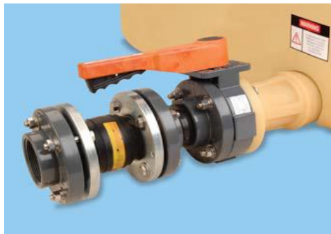
3" FDO (left) and 4" FDO (right) with flanged coupling, butterfly valve, and flexible expansion joint.
