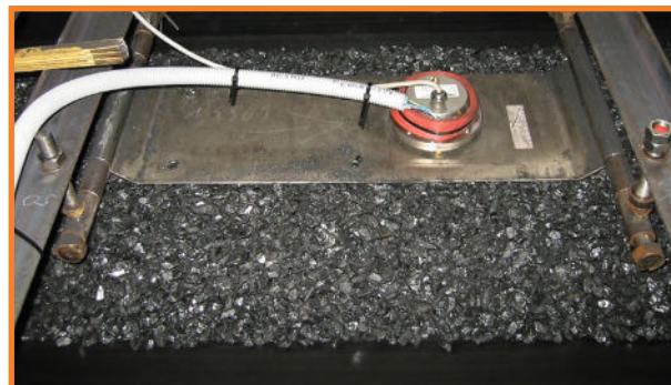
Measuring moisture of coal after the mill
