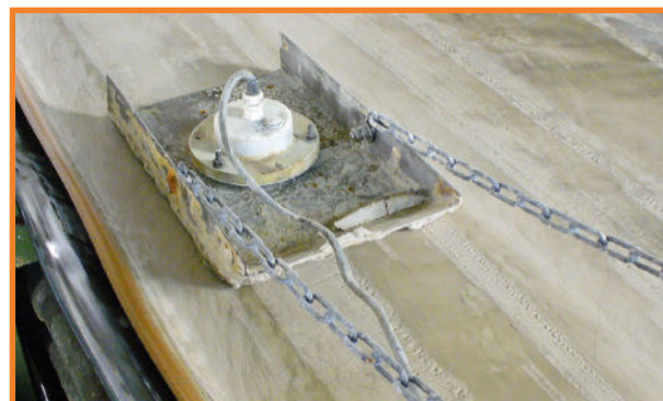
Measuring moisture of gypsum
