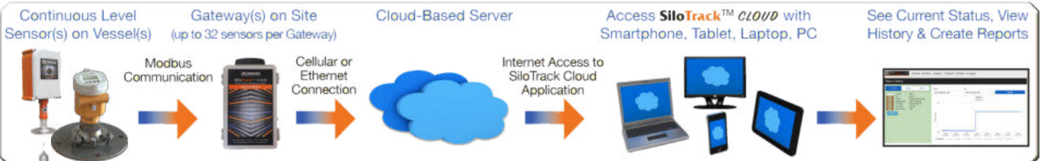
Durable Gateway for wireless or Ethernet connection to the Cloud-based server.
