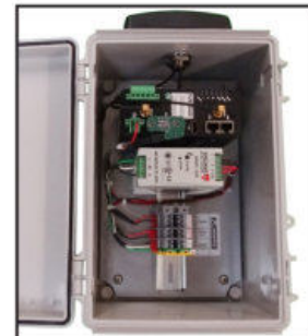
Durable Gateway for wireless or Ethernet connection to the Cloud-based server.
